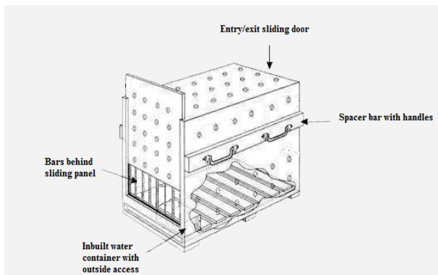
Figure 7. An example transport crate. Advice on specific requirements of crates for various wildlife taxa can be gained from speaking to in country rescue centers dealing with specific taxa.
